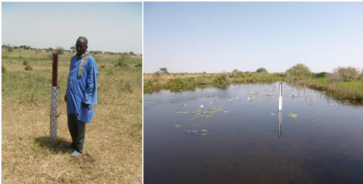
Left: In September 2011 there is no water at Pont Alain Daniel, just after the rains. The picture shows President Amadou Sow next to the scale at Pont Alain Daniel (PAD). Right: In January 2014 the same scale measures 40 cm of water.
