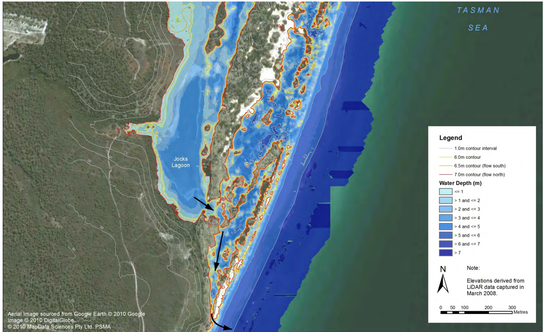
Figure 16: Water depths and topographic information at Jocks Lagoon (based on LiDAR projections). Note the areas to the east of Jocks Lagoon showing a water depth within the sand dunes are only indicative as these areas only hold water for short periods after flooding.
