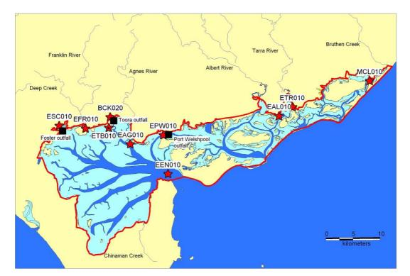
Figure 3-6 Corner Inlet Ramsar Site (red outline) with Locations of Waterwatch Sampling Sites (red stars) and Outfall Locations for Foster, Toora and Port Welshpool Wastewater Treatment Plants (black squares)
