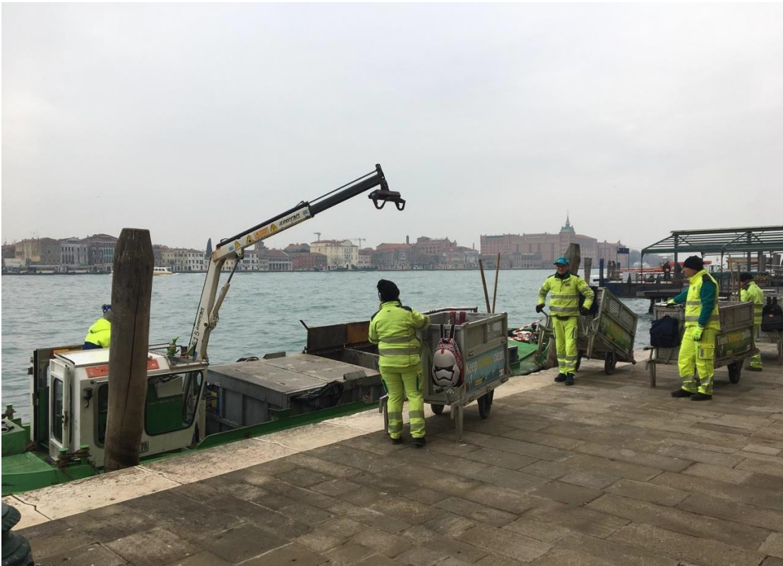
Urban Waste collected in differentiated small handcarts is reloading by crane into a hydraulic compact container on a ship. (Bernhard Furrer)
